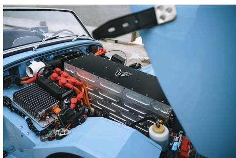
A stack of three Tesla batteries sit up front, and two more fit in the trunk. DW Burnett
