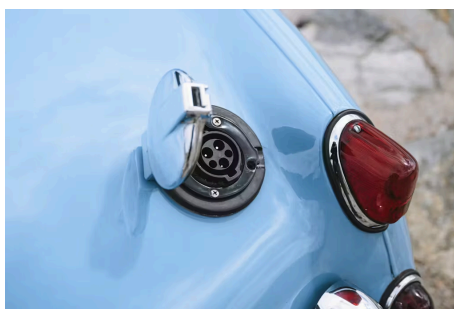
A 220V charger hides behind the original fuel filler cap. DW Burnett
